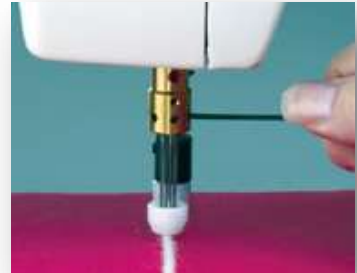
Close up of needles being changed
